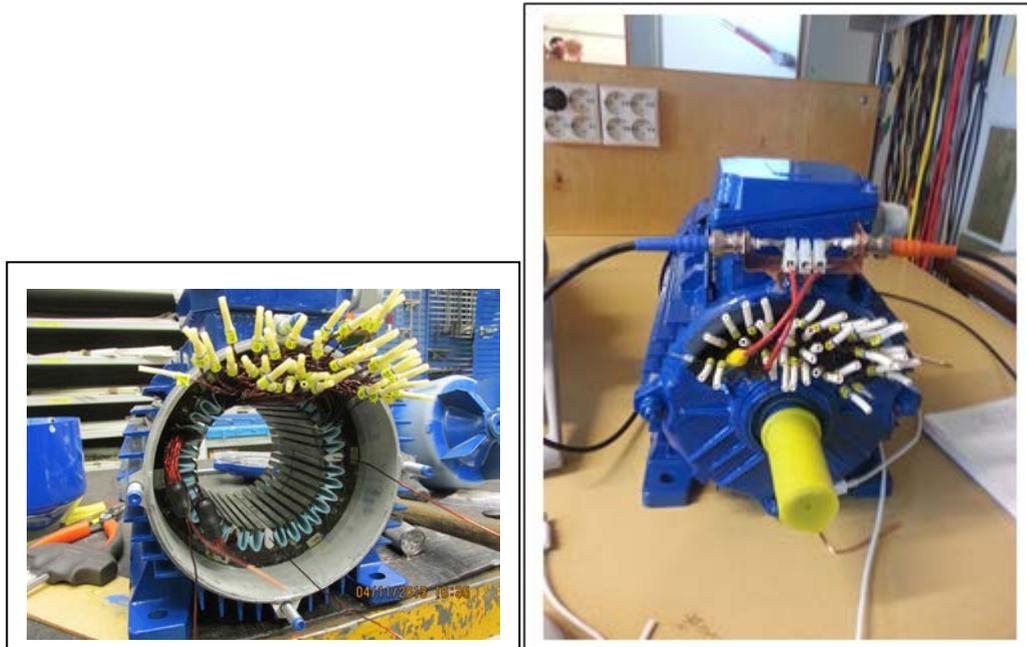
Fig. 3. Photographs of the built prototype with special windings
