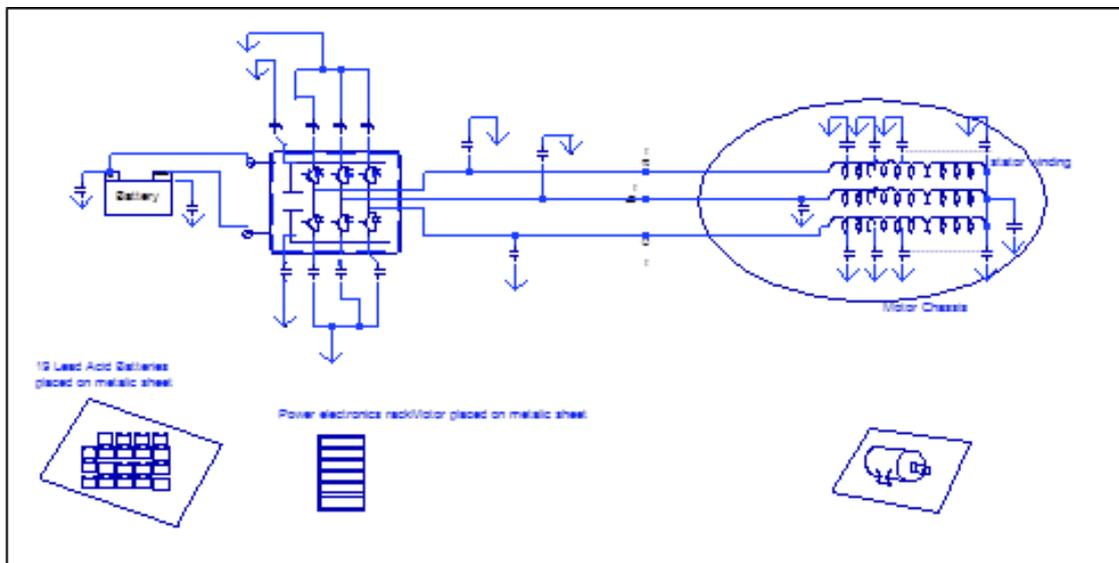
Fig. 2. Parasitic capacitances in an electric drive system
