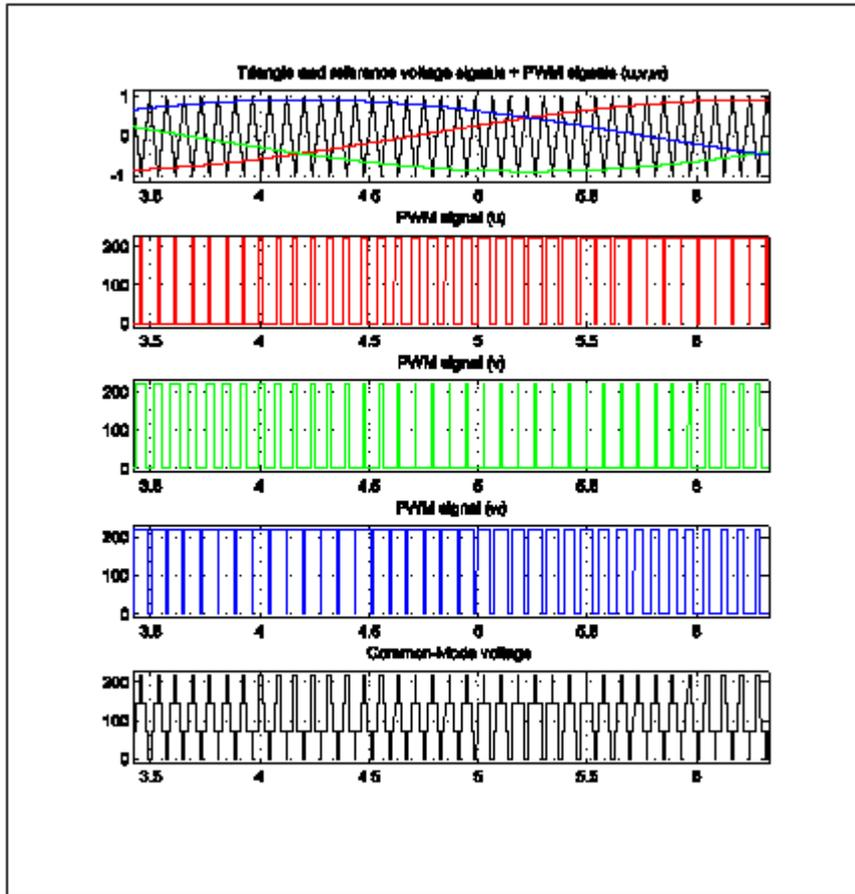
Fig. 1. Triangular wave modulation, PWM waveforms and common-mode voltage waveform.
