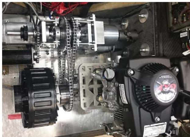
Figure 1 – Down-scaled experimental prototype of the hybrid-electric driveline configuration suggested in [1].
