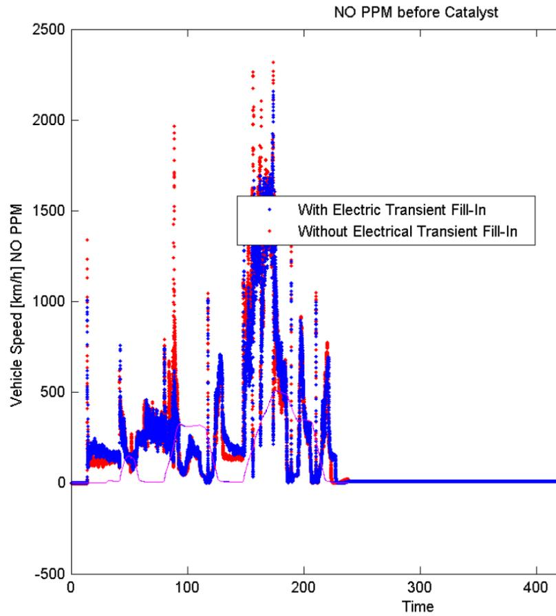
Figure 2. Engine out emissions (NO) before catalyst comparing strategies with and without electric torque fill-in
