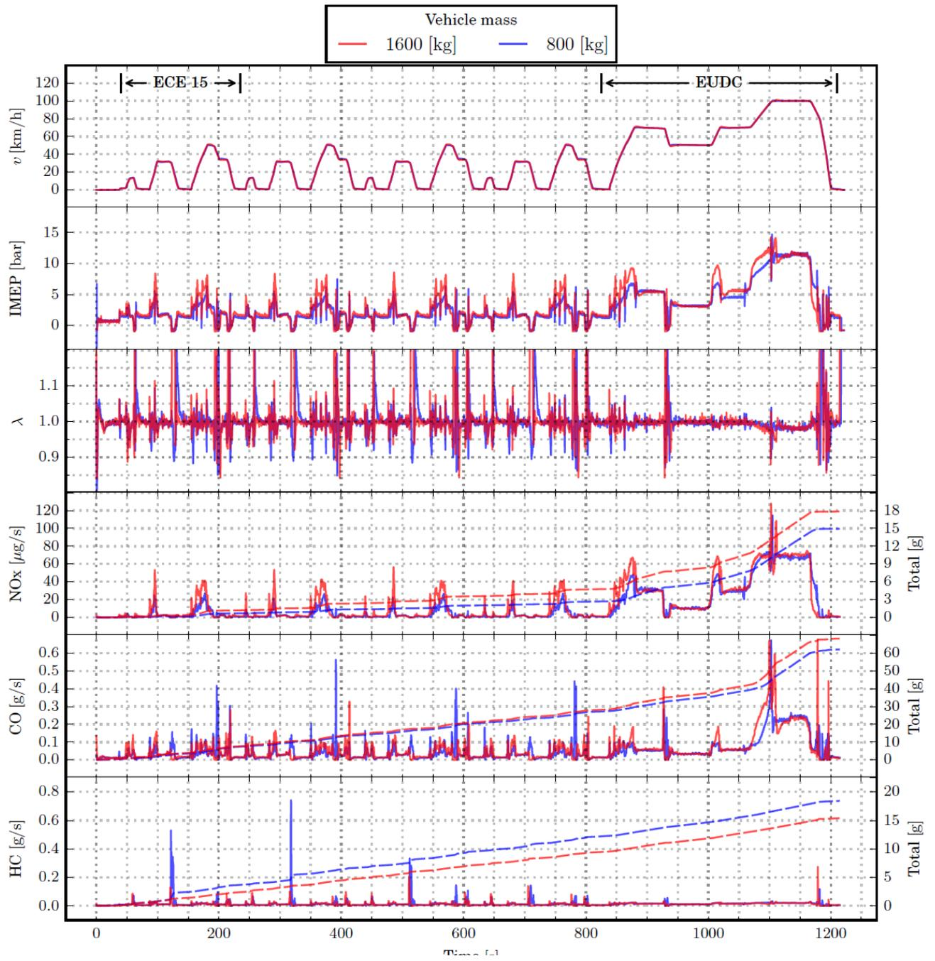
Figure 1 Representing a comparison between transient emissions tested with different vehicle mass. Solid line represents mass rates and accumulated emissions are represented as dotted lines in the figure.
