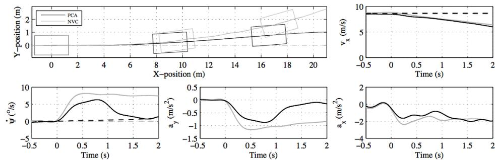
Figure 1. Measured vehicle trajectories and vehicle states for the vehicle with (PCA) and without (NVC) control strategy during failure condition.
