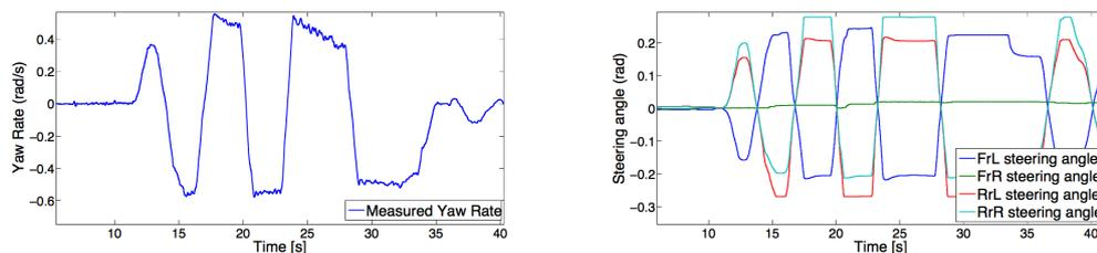
Figure 2. Yaw-rate response and steering angles for each wheel when deactivating the front right steering actuator.
