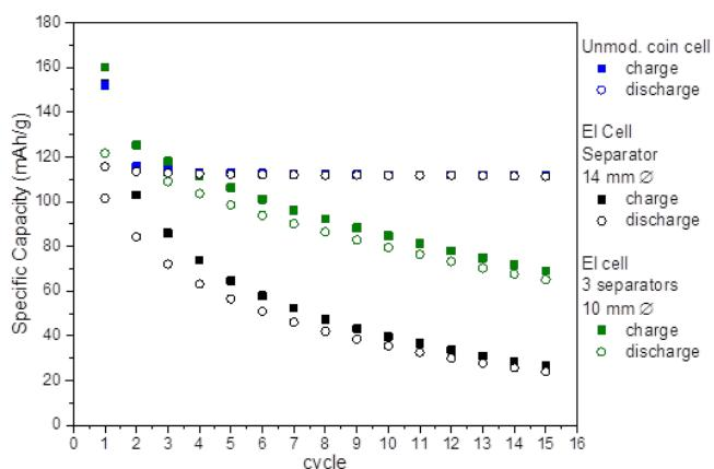
Some typical cycling performance is shown above. Interestingly our own set-up with modified coin cells performs better. However, for the acquisition of spectra the latter gives much better data and reproducibility (below shown for 3 unique grains of the negative electrode).
