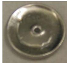
The modified coin cells (above) have been our own development for cheap and multiple analysis – but still has the problem of many failing cells – electrochemically.
