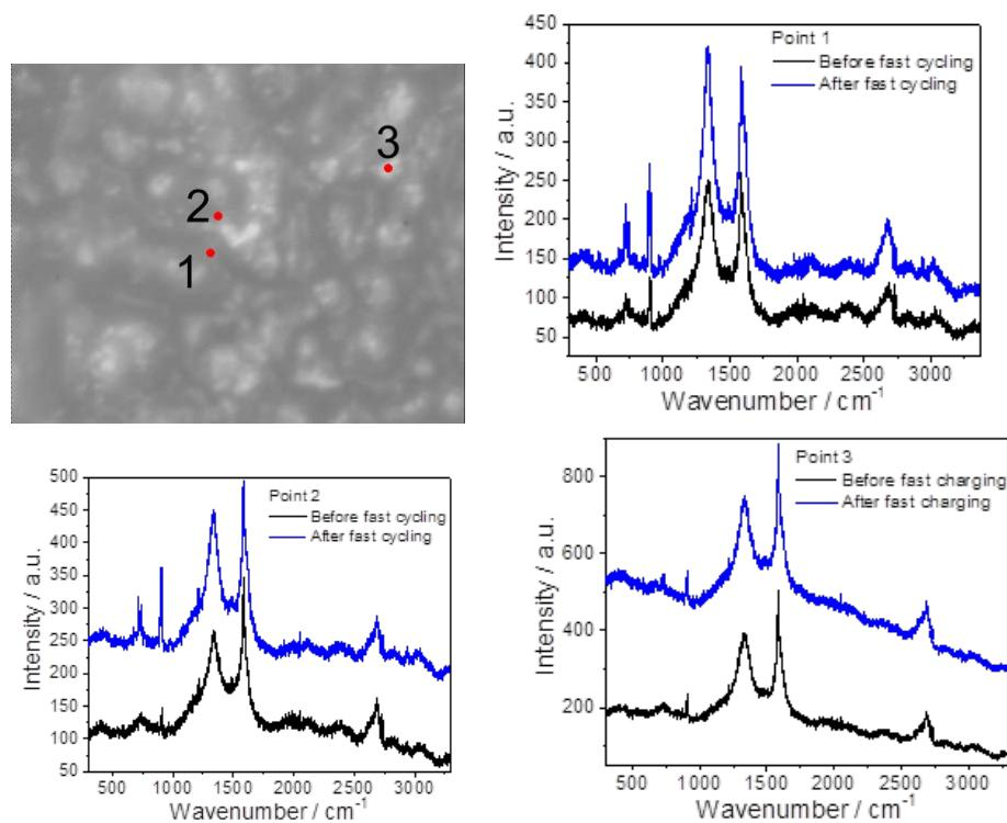
The typical spectra above focused on the first task: Can we see any unique degradation products on the surface when we are using a 4C-rate? Given that Raman *can* detect species at the ppm-level – the absence of any new features is indicative (and promising).
